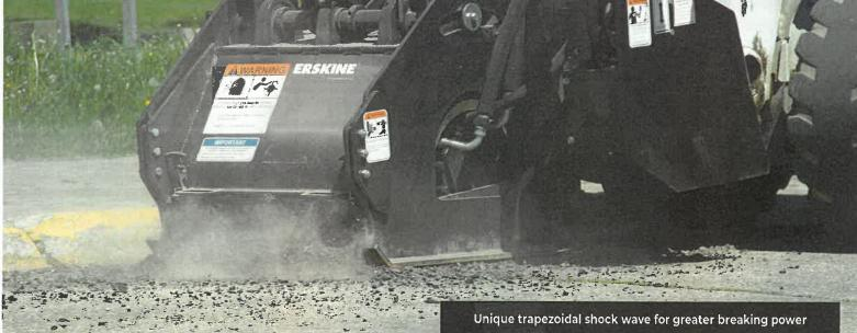
The Hydraulic Breaker makes quick work out of a tough job. The smart and efficient design provides a workhorse with only two moving parts. Vibration and shock are controlled by shock absorbing polymers, minimizing machine wear and sound while improving operator comfort level.
