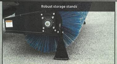
Oscillating design allows broom to follow uneven terrain
