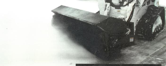
The Heavy-Duty Power Angle Broom design offers a heavy-duty frame, oversized bearing, and larger motor drive block. The strong and simple-to-use parking stands need no tools and have no pins that can get lost. The floating tilt follows the uneven surfaces for better bristle contact.
