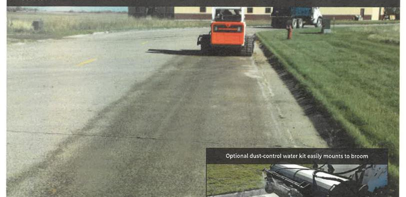
Sweep dirt and debris or scrape mud going forward. Ideal for construction, industrial or municipal jobs, it's easy to attach and simple to operate. The reversible cutting edge helps cut loose caked-on mud, while the sweeper's poly bristles deposit dirt and debris in the container.
