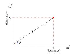
Figure 1: Impedance vector: Real and Imaginary components
