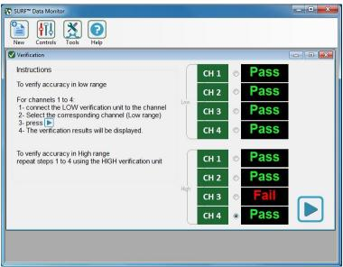
Figure 35: Device verification results
