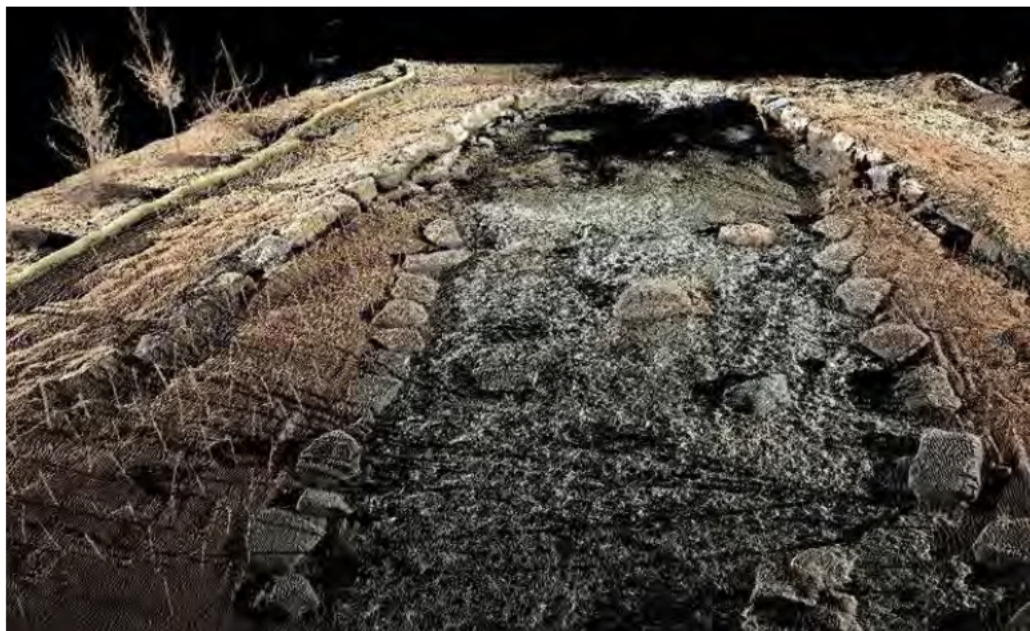
3D As-Built Scan of a Cross Vane
