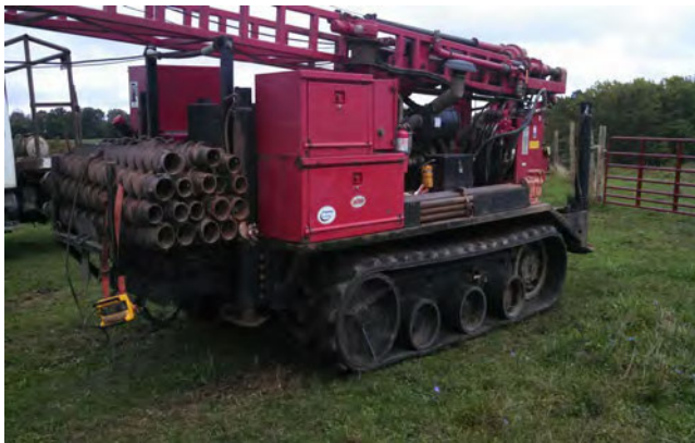
Diedrich D-50 Rubber Track Mounted Drill Rig
