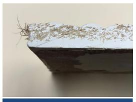
Plaster sample with gypsum and coconut fibers
