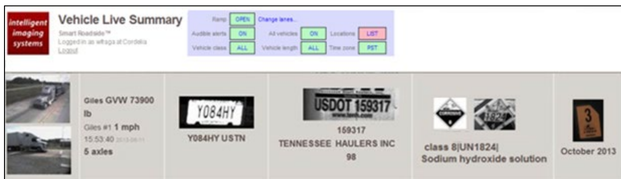
Figure 4: Example of single vehicle digital file summary display including CVSA decal information
