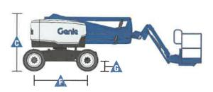
The metric equivalent of working height adds 2 m to platform height. U.S. adds 6 ft to platform height.
