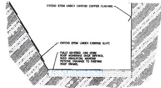
**TYPICAL ROOF EDGE AT COPPER FLASHING DETAIL**
