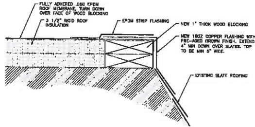
**TYPICAL ROOF EDGE AT SLATE ROOFING DETAIL**
