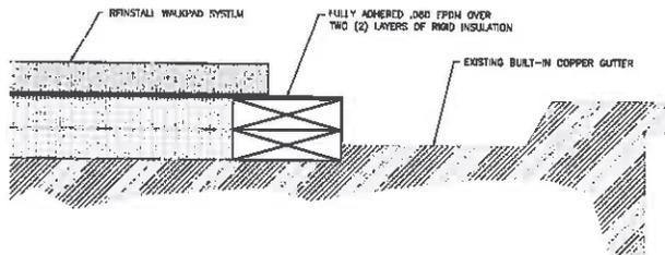
**TYPICAL ROOF EDGE AT BUILT IN GUTTER DETAIL**
