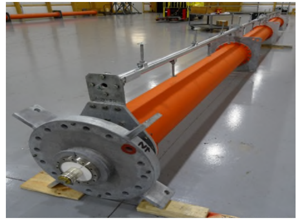
Top mounted TRASAR with galvanized steel climbing pole used with horizontally polarized and directional circularly and elliptically polarized antennas.
