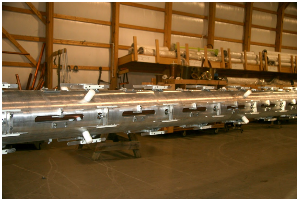
ERI elliptically polarized side mounted UHF television antenna under construction. The slots shown provide the horizontally polarized signal and the vertical dipoles between the slots emit the vertical signal component. This allows the horizontal plane patterns of the two polarizations to be optimized for the best over the air coverage for any given location and application.
