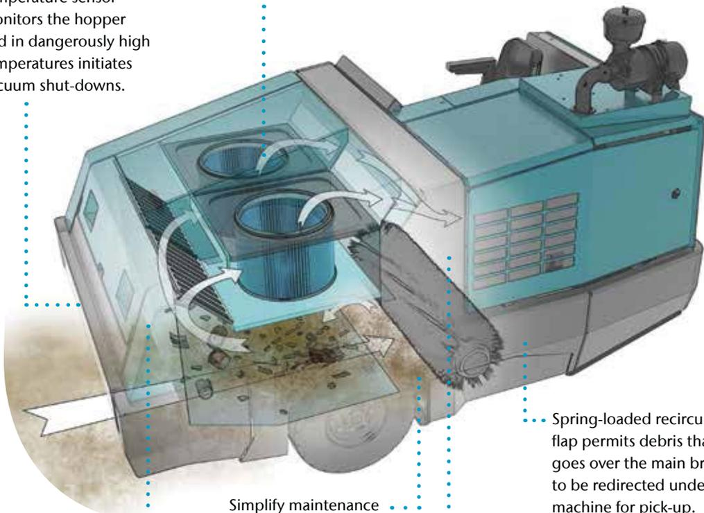
Multi-level dump hopper empties debris into containers as high as 6 ft / 1.8 m.
