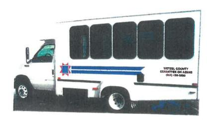
158" Wheelbase Cutaway Vehicle (Paratransit)
