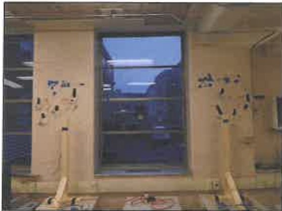
Instrumentation to evaluate clay tile walls Hodges Hall, WVU
