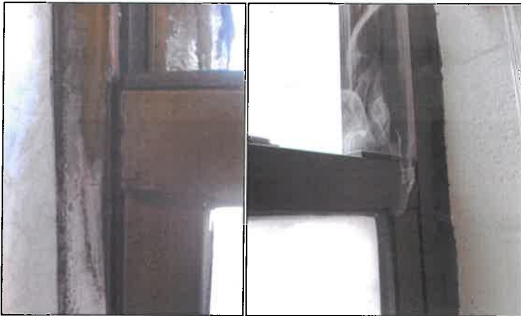
Left: Reported Ice Lensing on Interior Side of Window Frames Right: Smoke Pencil Testing for Air Leakage at Windows
